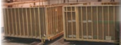
Electric is run and the insulation is installed. The home is sheathed, wrapped with Tyvek, then the windows and siding are installed.
